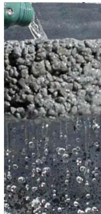
Infiltration capability of porous pavement Photo by Greg McKinnon from Puget Sound Online
